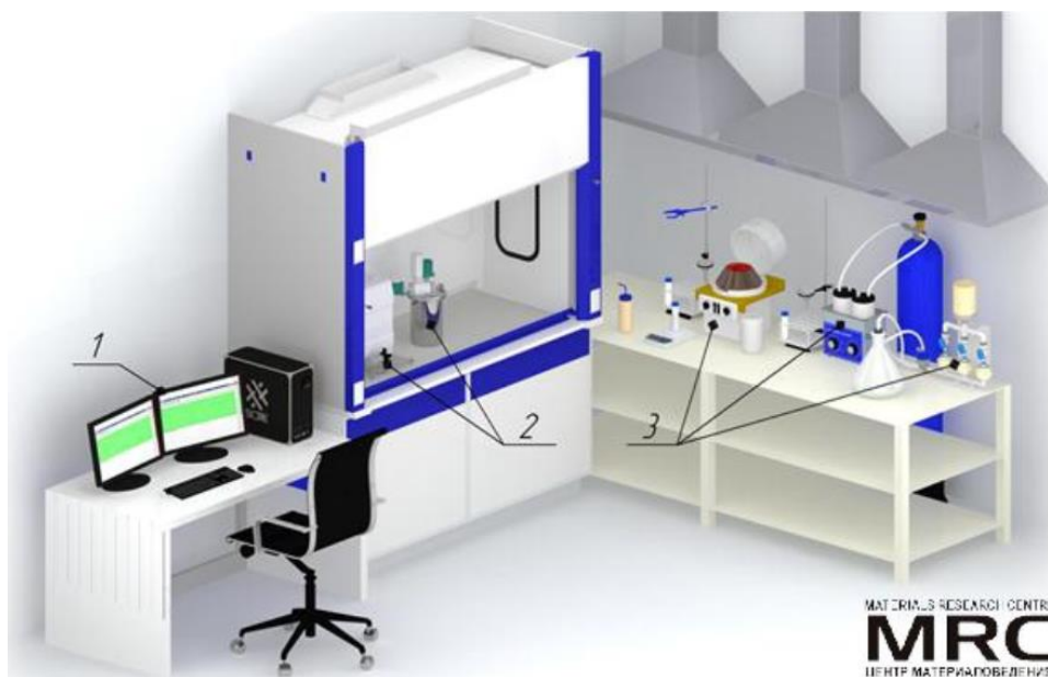
Fig. 1. Pilot laboratory line with controlled parameters for MXene synthesis (up to 100 g per batch): 1 – computer control system; 2- Etching reactor for MXene synthesis; 3 – additional equipment for laboratory technological line.
